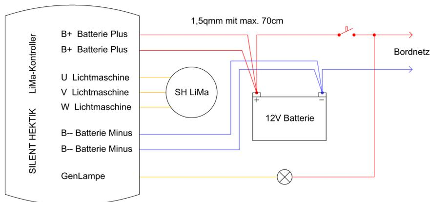
The minus plug which connects the alternator controller and the battery is obligatory!
