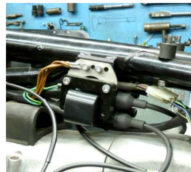
The distance from the box to coils should be min. 10cm
